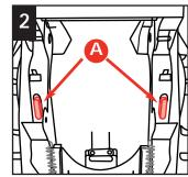
Adjust backrest to lowest position. Remove both lower harness guides (A) in bottom of seat under recline stand.
